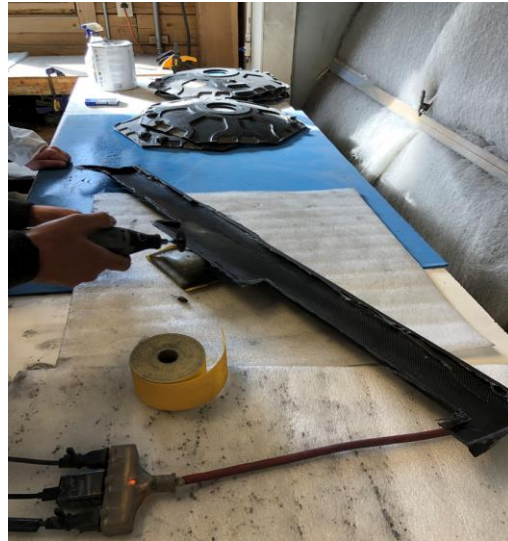
Figure 26: Trimming with Dremel
