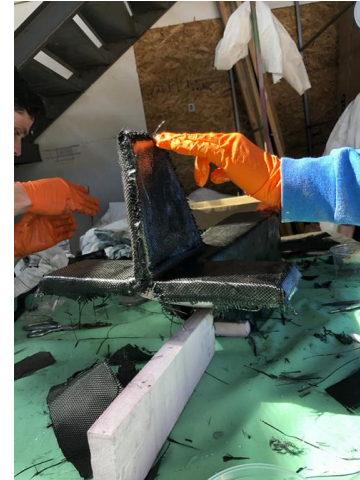
Figure 29: Wet layup of Fuselage
