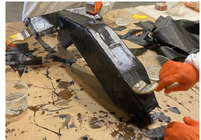
Figure 35: Fuselage Wet Layup
