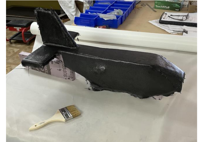
Figure 34: Fuselage Wet Layup
