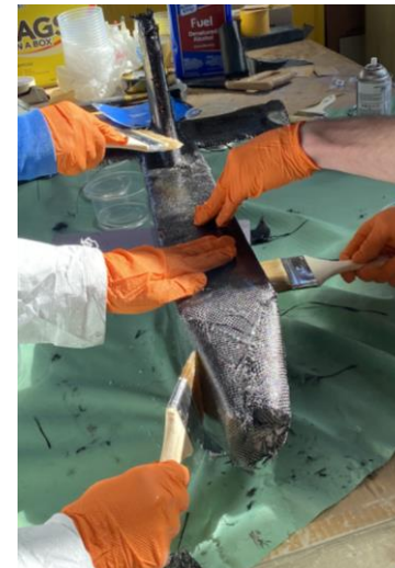
Figure 31: Wet layup of Fuselage
