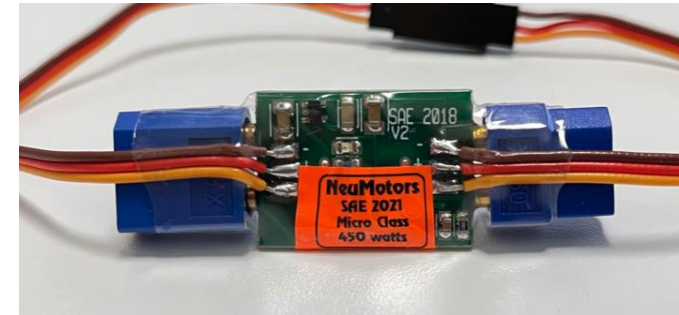
Figure 12: Neumotors SAE Power Limiter [6]
