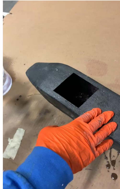
Figure 33: Removing Foam with Acetone
