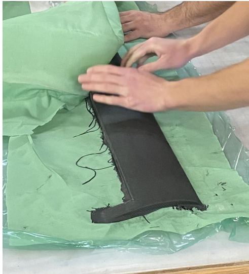
Figure 25: Removing Part from Vacuum Bag
